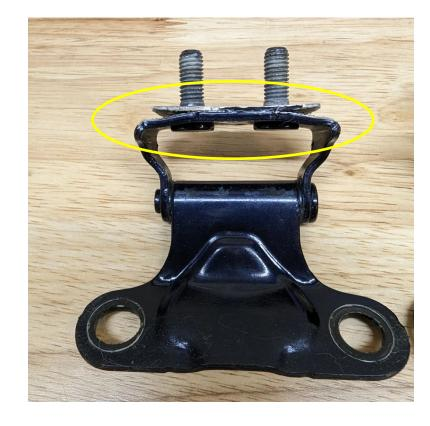
57. As such, when Plaintiff and the Class attempt to use the power liftgate, the hinges fail to operate correctly and will separate from their intended place on the body of the vehicle and begin to tear apart, which causes further damage to additional areas that surround the hinges, including the paint and body.
