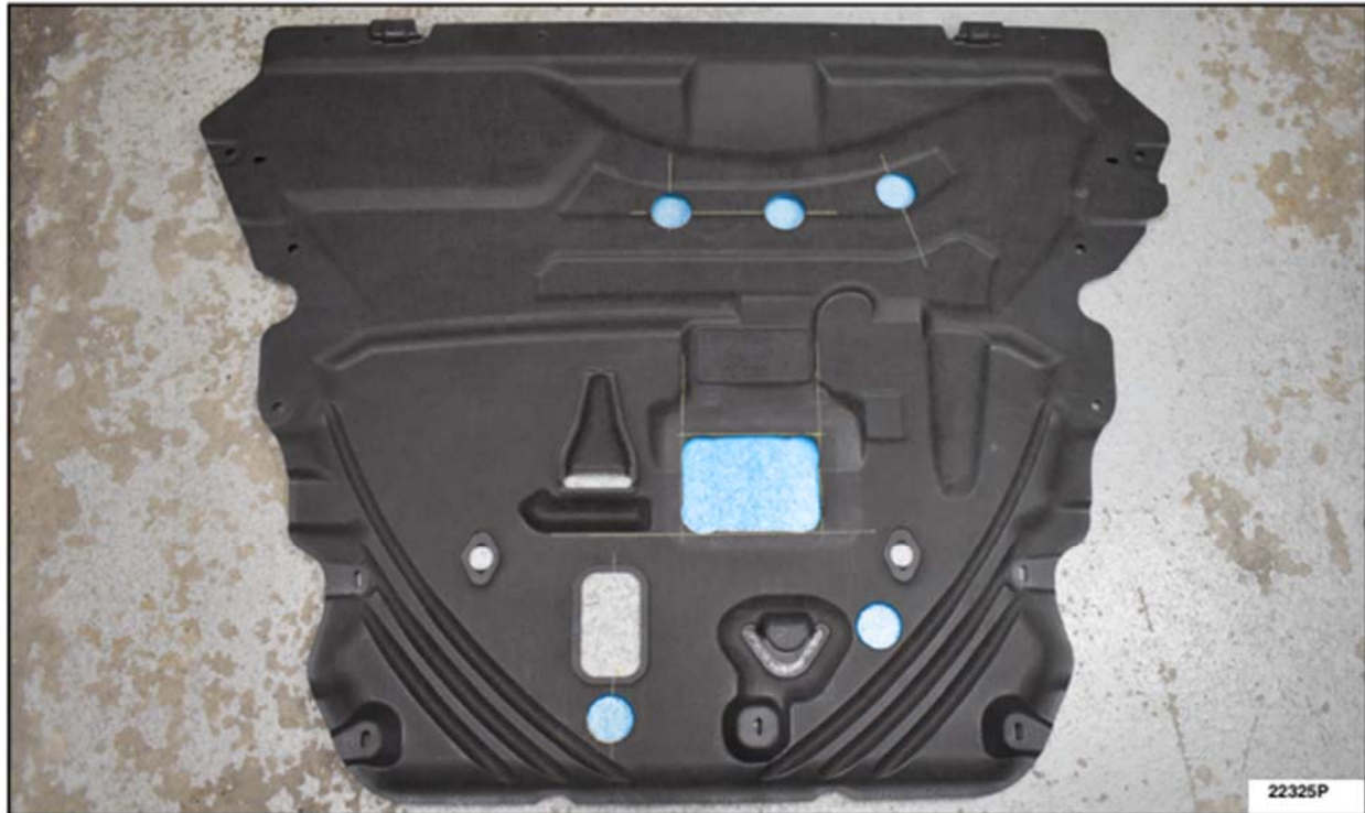
Figure 1: Image from Ford’s letter to its dealers demonstrating the under engine shield modification, with additional drainage holes highlighted in blue, as part of the required “fix” on all Spontaneous Fire Vehicles. 8
