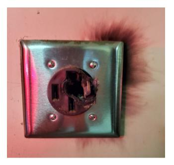
33. Similarly, on or about January 3, 2023, another Taycan owner found that the included supply cable, plugged into a NEMA 14-50 outlet, had melted both the outlet and the cable's plug<sup>:28</sup>
